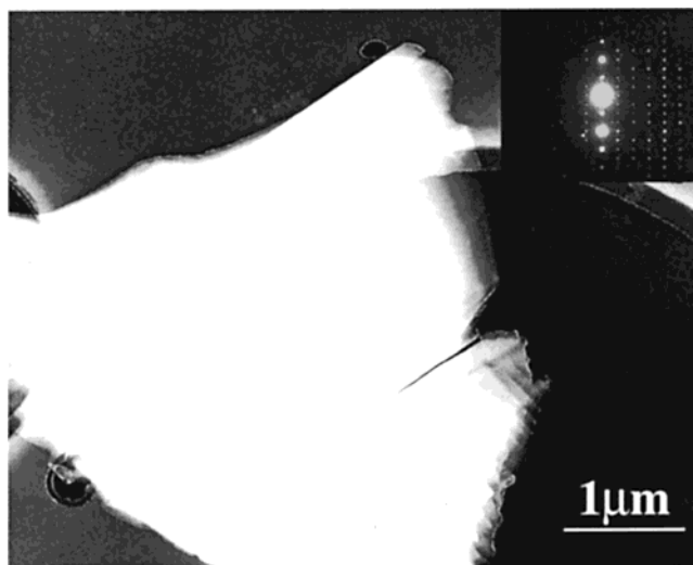
Figure 5. TEM pictures, showing the morphology and the diffraction pattern (the insert) of a typical crystallite of the annealed \text{C}(\text{DPVBi})_4 .
